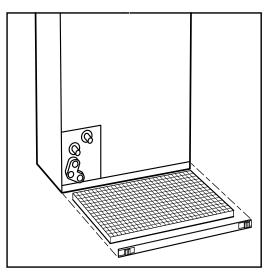
Fig. 5—Removing Filter from Fan Coil Unit
